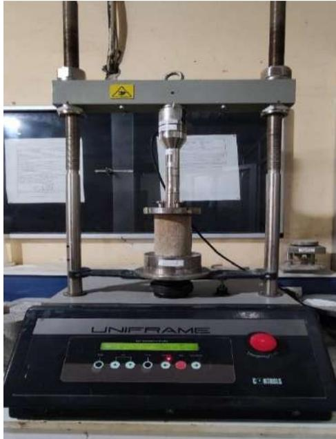
**Figure. 5.** Unconfined compression tests of the specimens.
